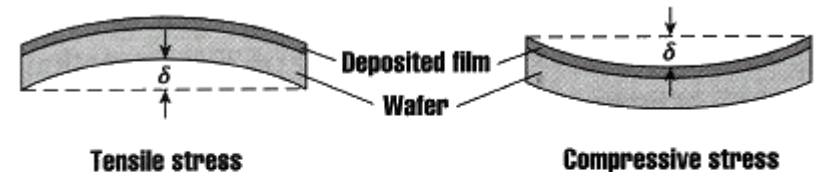
Figure 12-28 The change in wafer deflection may be used to measure the stress in a deposited layer. This is typically measured using a reflected laser beam.
